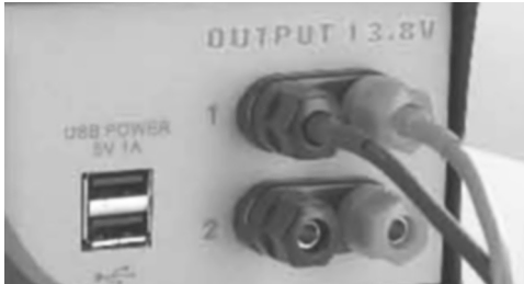
4mm bullet connectors plug directly into most power supplies.
