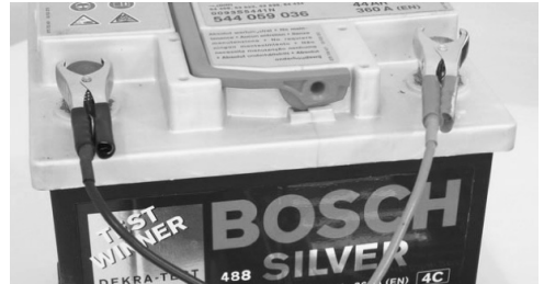
Using terminal clip attaching to car battery.
