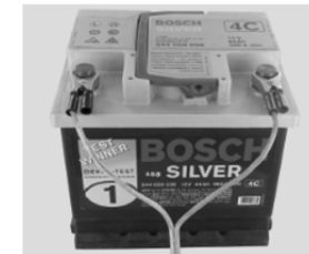
Using DC cable attaching to car battery
